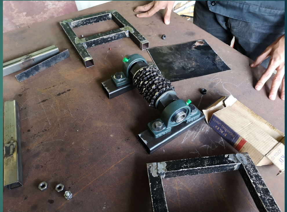
Innovation of the blade which is the main part to do breakdown process of the raw kulit durian
